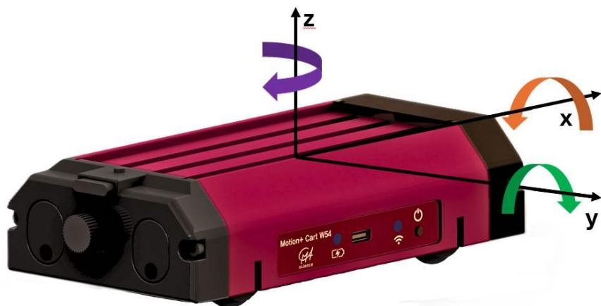
This is achieved using a 3-axis gyroscope, which detects changes in angular position by measuring the rate at which the cart's orientation changes over time. As the cart rotates, the gyroscope senses the angular motion and translates it into electrical signals, which are then processed to give accurate readings of the angular velocity in each direction. This allows precise monitoring of rotational movements and helps in studying rotational dynamics and angular motion in physics experiments.
