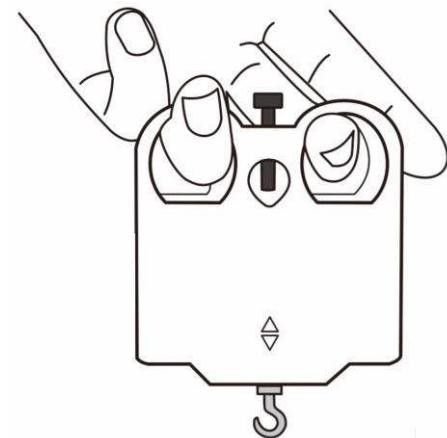
Since the 3-Axis Accelerometer is equivalent to three accelerometers, you can use just one channel of it to study acceleration along a single axis. Mount the accelerometer so that a particular axis is in the direction of interest and monitor just that channel.
