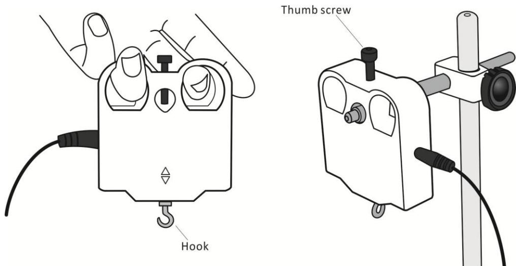
To zero the measurement of the force sensor double press the power button. Do it again to return to the normal measured value.
