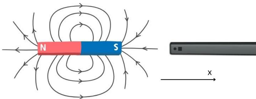
The measurement in the x-direction is positive when the South pole of a magnet is located in front of the wand and the Hall element, pointing in the x-direction, as shown in the image above.
