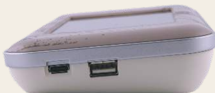
USB C port (left) for charging and communication USB port (right) for connecting any USB peripheral
