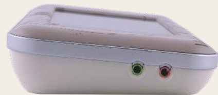
Audio Out (left) for generating DC/AC voltage signals Audio In (right) for connecting external microphone
