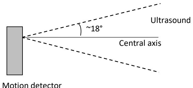
The sensitivity of the echo detection circuitry automatically increases as the ultrasound travels outward. This is to allow the detector to pick up weaker echoes from distant objects. For accurate measurements the object should have a flat front perpendicular to the line between sensor and object.
