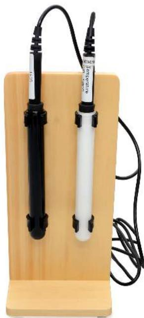
The graph below shows an example of measurement results. A strong halogen lamp is used to heat the empty black and white tubes as shown on the photo below.
