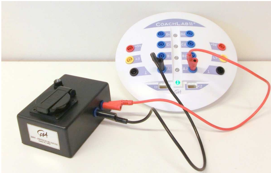
Figure 2. Connecting the switch module to the CoachLab II + interface.
