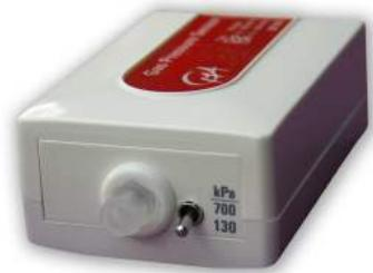
The pressure is measured via a pressure port located next to the switch. The pressure port has a small threaded end called a *Luer-lock*. With a gentle half turn, you may attach a plastic tube or a valve with Luer-lock connectors. You can also attach the 20-ml plastic syringe included with the sensor directly to this port.
